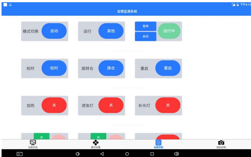
After entering manual mode, the light control, rain control, and time control will not be triggered. You can manually control the operation of each component. Manual mode is intended for debugging purposes only, and it is advisable to avoid using it if you are not familiar with the device.
