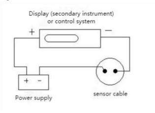
(1) If the sensor outputs other signals, the conventional sensor line sequence and function correspondence are as follows:
